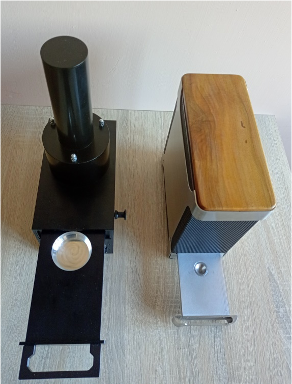
Figure S3. Photos of OSL Helios and SUERC readers with visible sample holders/drawers.
