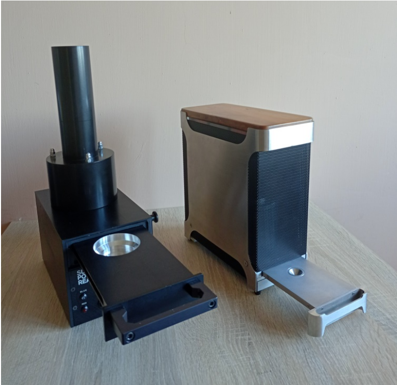
Figure S3. Photos of OSL Helios and SUERC readers with visible sample holders/drawers.
