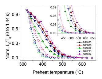
**Fig. 5.** Pulse anneal curves for pIRIR(50,290) stimulation for samples 951020 (squares), 963806 (circles), 951912 ("upright" triangles), 062213 ("down" triangles) and 981014 (diamonds). Also shown are the pulse anneal curves for IR(50) (open symbols and dashed lines). The inset shows a close up of the data.
