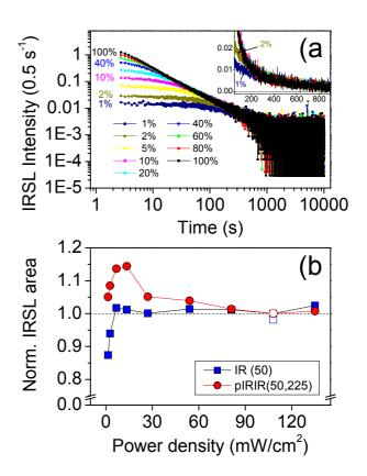
**Fig. 8.** a) Effect of changing the stimulation power on decay shape for the IR(50) signal from sample 981014. A background using the last 5 s of stimulation has been subtracted and the curves have been corrected for sensitivity change (see text for details). The inset shows a close up of the data. b) The area of the individual decay curves for a constant number of incident photons as a function of incident power for the IR(50) and pIRIR(50,225) signals.
