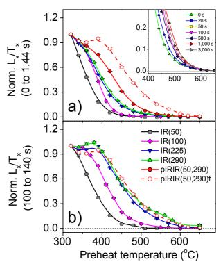
**Fig. 4.** Pulse anneal curves for sample 981014 for IR(50), IR(100), IR(225), IR(290) and pIRIR(50,290) for 100 s of prior IR(50) stimulation. a) Initial signals (first 1.44 s). Also shown is the final signal for pIRIR(50,290) stimulation (pIRIR(50,290)); dashed line). The legend is given in b). The inset shows the effect of changing the stimulation time of the prior IR stimulation in the pIRIR(50,290) signal. b) Final signal (100-140 s).
