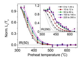
**Fig. 3.** Pulse anneal curves for IR(50) measured for 1,000 s for different summation intervals down the decay curve of sample 981014. The data have been normalized to the initial preheat temperature of 320°C. Legend is given in the inset, which also shows the pulse anneal curves obtained for IR(290) measured for 400 s. The dashed lines in the inset are the pulse anneal curves for the initial and final IR(50) signals.
