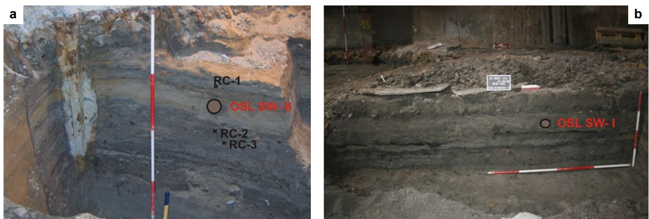
Fig. 2. Sampling points for OSL samples SW-II and SW-I. For SW-II material was taken from an intercalated fluvial sand layer. From the more heterogeneous material from above and below the sand layer, material for radiocarbon dating was taken (samples RC-1, RC-2, RC-3). Sample SW-I was taken in a distance of about 5 meters west from SW-II. The strong deformation structures around SW-I were assumed to have been caused by anthropogenic movements in shallow water.
