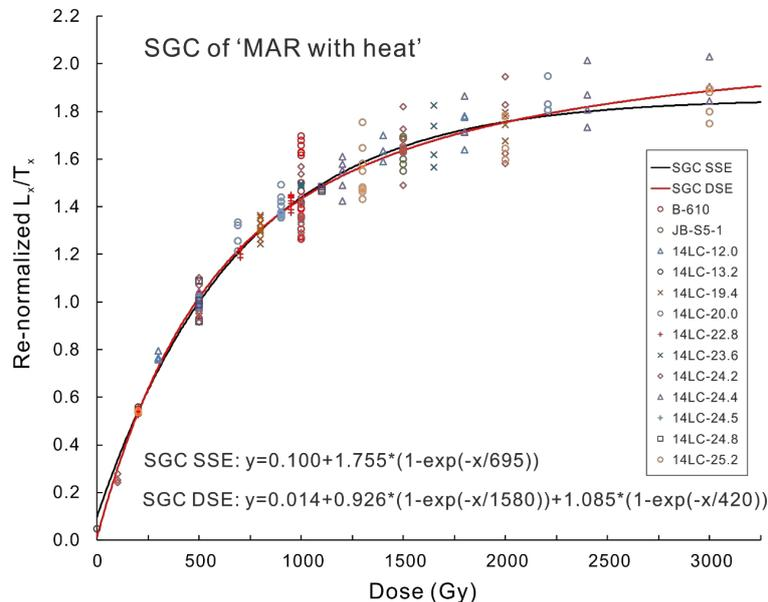
Fig. 3. Standard growth curve (SGC) of the 'MAR with heat' protocol. The re-normalisation dose was 500 Gy. SGC curves were fitted with the single saturating exponential (SSE) function:  $y = y_0 + A \cdot (1 - \exp(-x/D_0))$  and the double saturating exponential (DSE) function:  $y = y_0 + A_1 \cdot (1 - \exp(-x/D_1)) + A_2 \cdot (1 - \exp(-x/D_2))$ , respectively. The fitted results are shown in the graph. Note that the two SGCs only begin to diverge when the dose exceeds 2000 Gy.
