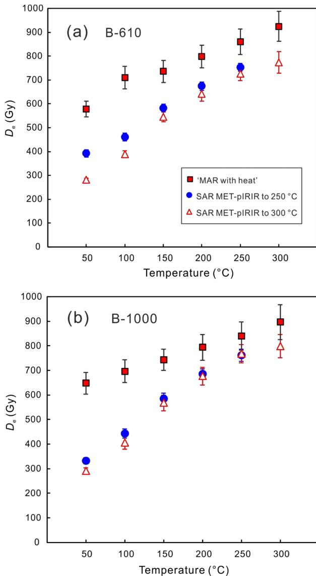
**Fig. 5.**  $D_e$  values with different stimulation temperatures for the two SAR protocols with MET-pIRIR stimulation to 250  $^{\circ}$ C or 300  $^{\circ}$ C, and the 'MAR with heat' protocol. Note that the MAR  $D_e$  values always exceed the SAR  $D_e$  values.
