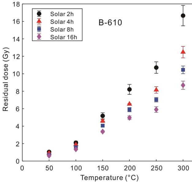
Fig. 2. Residual doses of IRSL signals stimulated at different temperatures using the SAR MET-pIRIR protocol. After 8 hr of bleaching with the solar simulator, the residual doses were reduced to ~10 Gy for the MET-pIRIR<sub>300</sub> signal.
