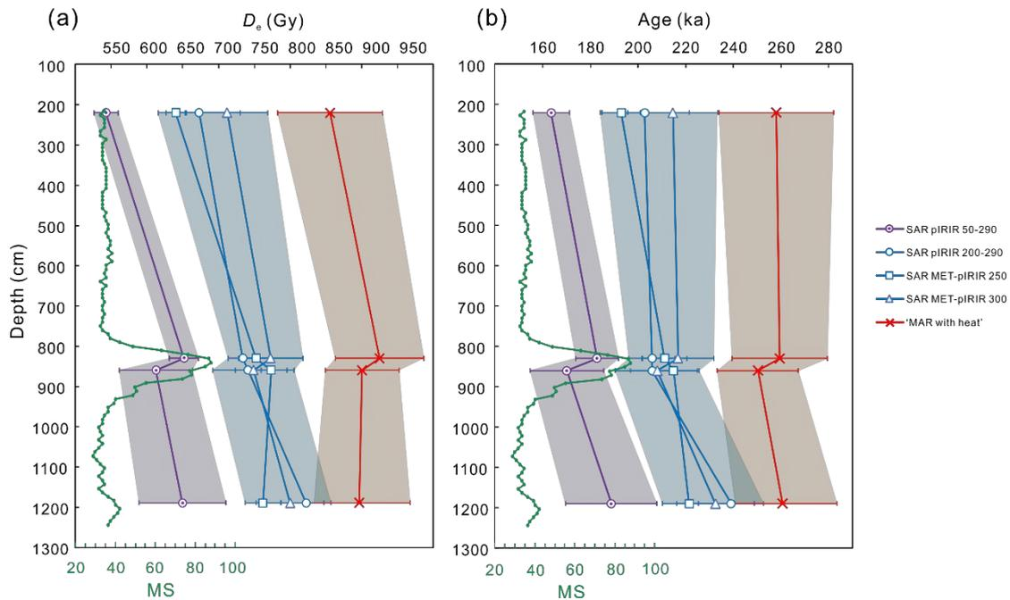
**Fig. 4.**  $D_e$  values and age versus depth relationship for section B. The SAR pIRIR<sub>50/290</sub> protocol has the youngest ages; the SAR pIRIR<sub>200/290</sub>, MET-pIRIR<sub>250</sub> and MET-pIRIR<sub>300</sub> protocols have similar ages; and the 'MAR with heat' protocol has the oldest ages.
