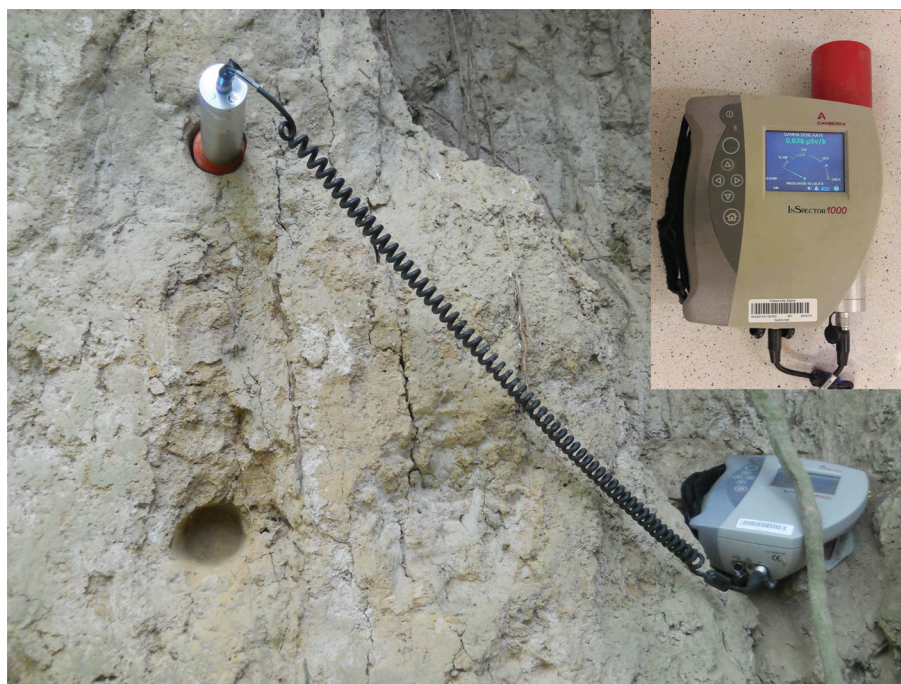
Fig 9. Portable scintillation spectrometer used during field measurements.
