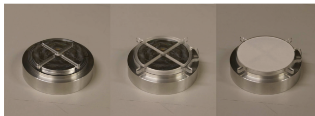
Fig 7. Sample holder for standard size 3 g samples prepared for measurement on the \mu Dose system.
