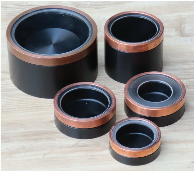
Fig 4. The new type of containers (gBEAKERs) for samples used in High-Resolution Gamma Spectrometry (HRGS) was developed in GLL (Poręba et al. , 2020). GLL, Gliwice Luminescence Laboratory.
