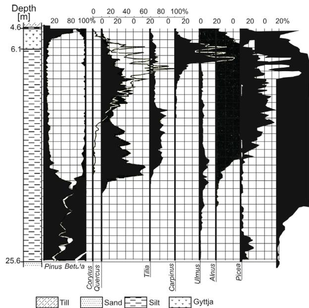
**Fig. 9.** Spore and pollen diagram of the interglacial sediments in the Snaigupėlė outcrop (Kondratienė, 1973).
