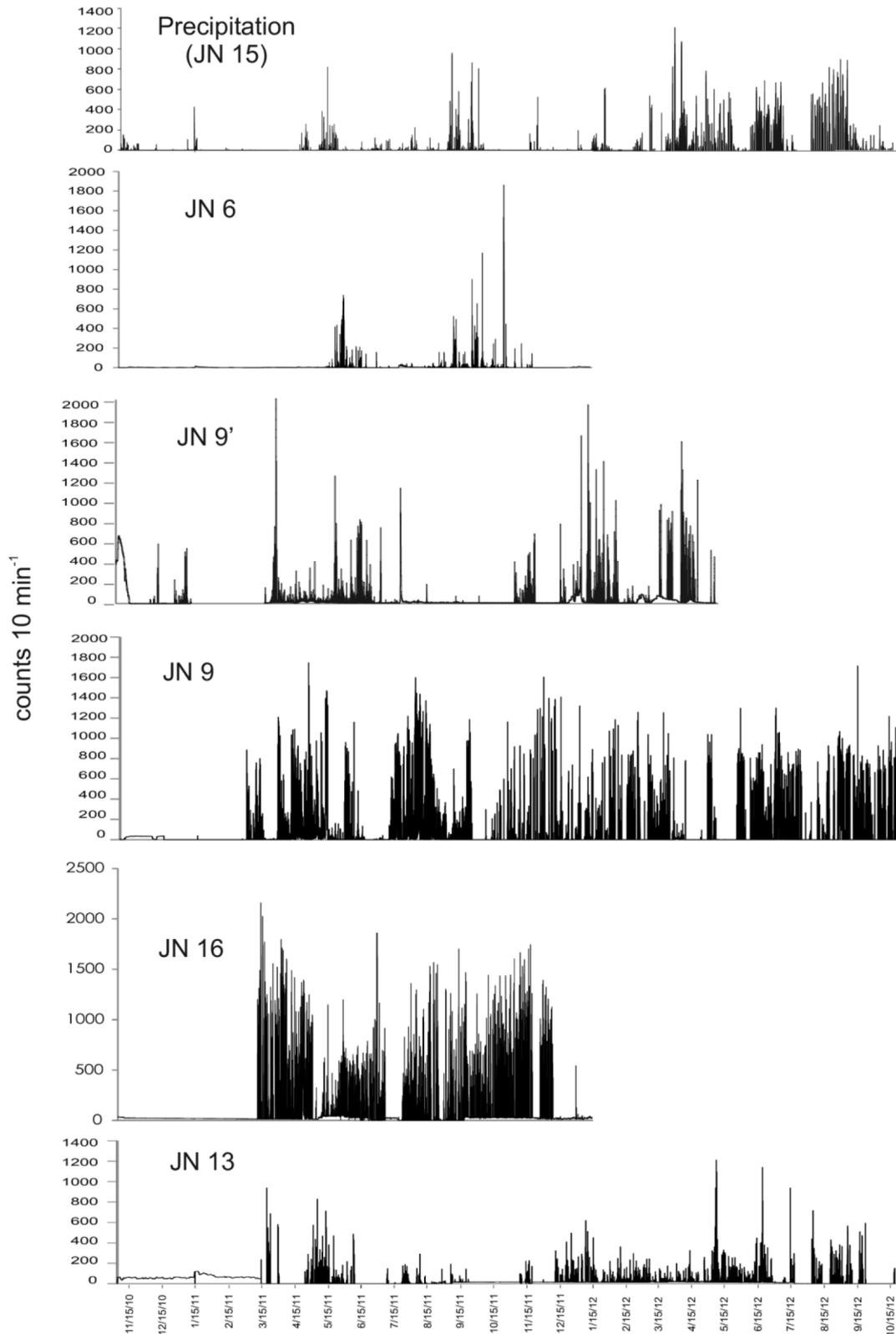
**Fig. 2.** Frequency and intensity of precipitation (JN15; upper graph) and changes in discharge (counts per 10 minutes) of studied drip points inside the cave. Site codes similar to these in the Fig. 1. Horizontal scale (time) is the same for all graphs.
