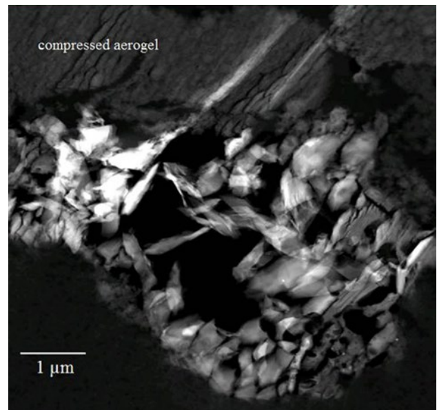
Fig. 9. Refractory grain collected from Comet Wild 2 by the Stardust spacecraft. Refractory minerals tend to be strongly thermoluminescent (Fig. 8), but in the case of the refractory mineral forsterite the luminescence fades rapidly in the presence of a few mol % Fe. (Geake et al. , 1973).
