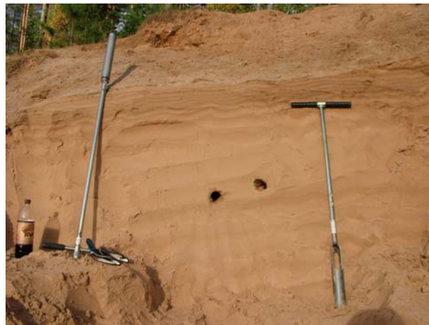
Fig. 3. Sampling of shallow water glaciolacustrine fine grained sand at the Pentsils site, 4 km proximal to the recessional moraine of the North-Lithuanian phase, 10 km WNW of the Valka/Valga Town. All the samples used in this study were collected in opaque PVC tubes, driven into cleaned, horizontal sediment sections. All sample collection was conducted under a black tarp to prevent light exposure sections of sample tubes.
