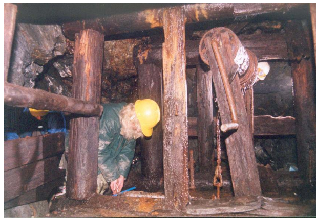
Fig. 3. Taking samples with the Pressler increment borer from the shaft timbering in the Marcinków mine.
