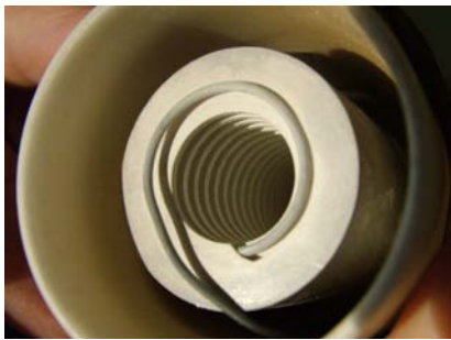
Fig. 1. The heater assembly made of molybdenum wire shaped into a helix, which is placed in the boron nitride ceramic insulator.
