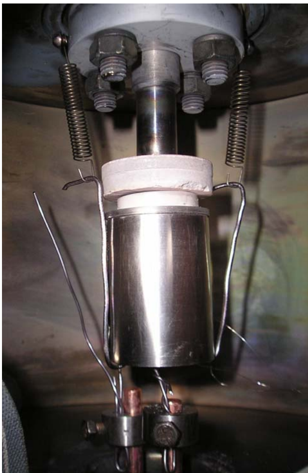
Fig. 2. The crucible with the heater.
