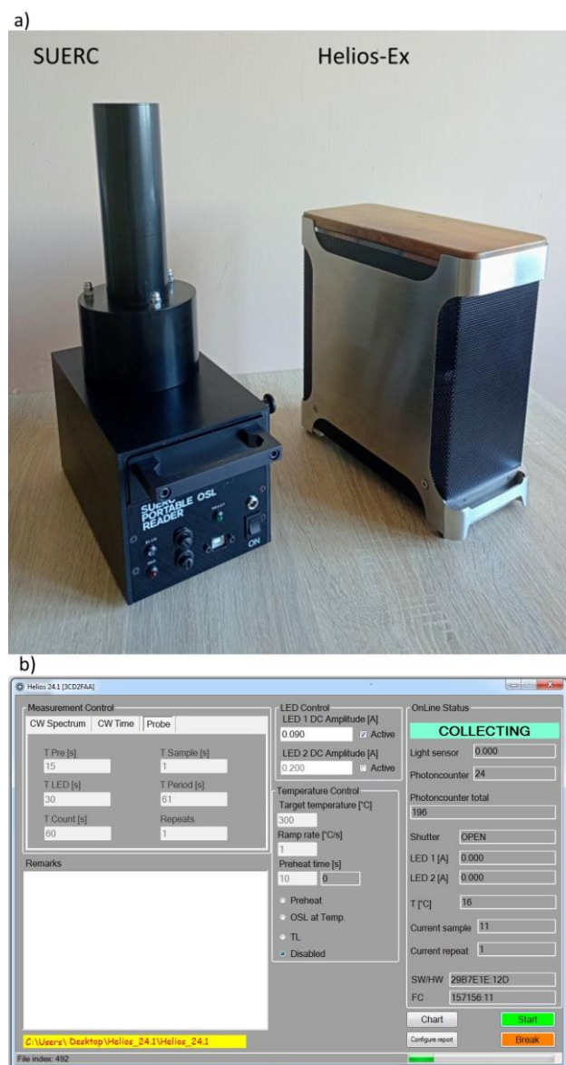
Fig. 1. (a) Photo of SUERC (left) and Helios (right) readers for dimension comparison only; (b) Screenshot of Helios control software (v24.1). Helios's dimensions: length: 245 mm, width: 110 mm, height: 260 mm, weight: 4.8 kg.
